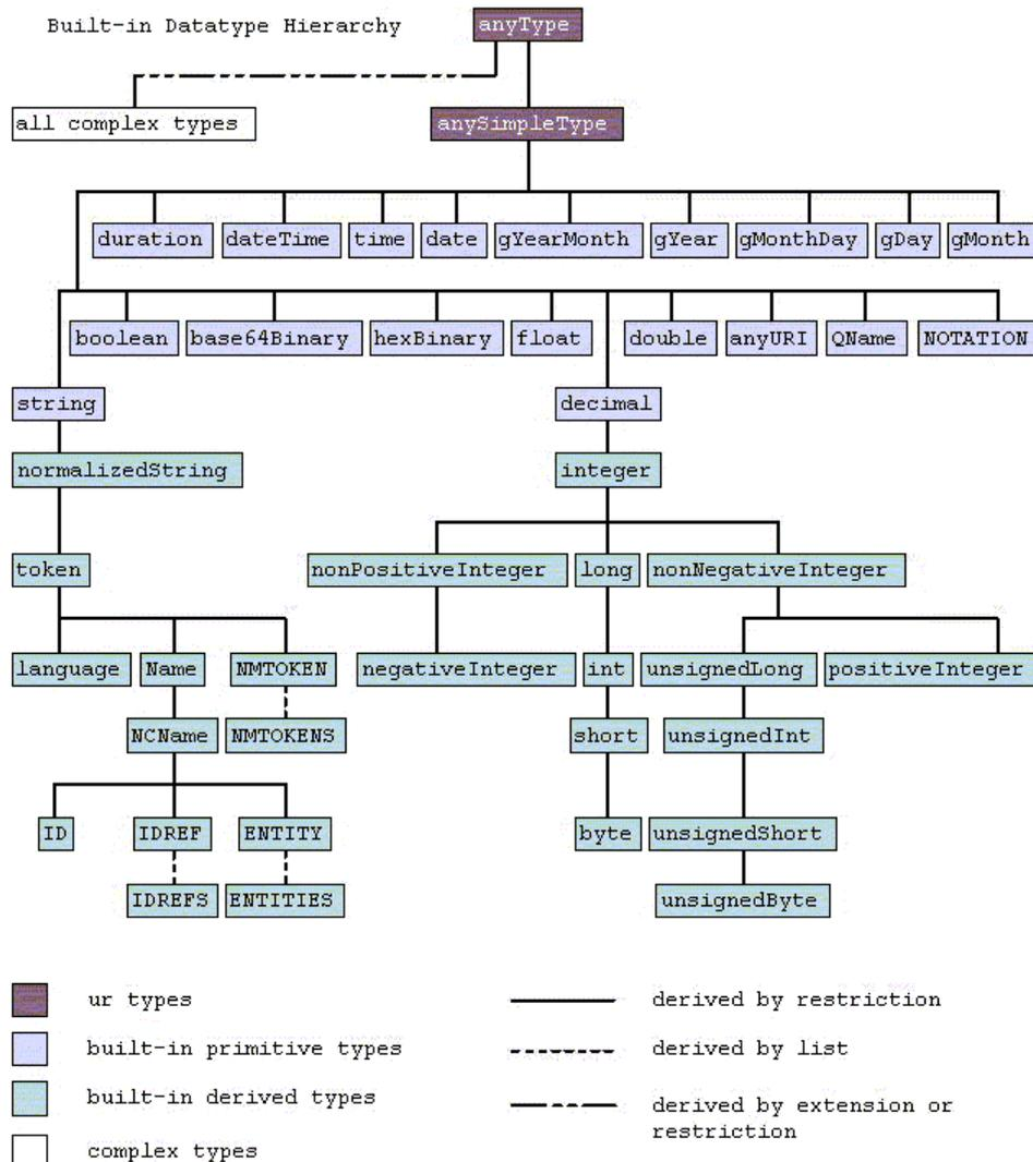
Figure 1: XSD types from W3C XML Schema [i.40]
